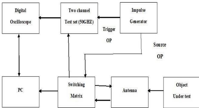
**Figure.10. Block diagram of UWB tomography system**
