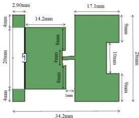
Figure.2. Geometry of proposed Patch antenna 1
