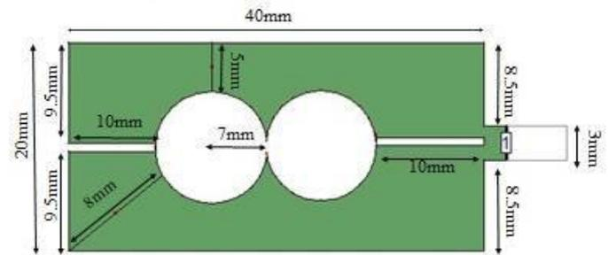
Figure.4. Geometry of proposed patch Antenna 2
