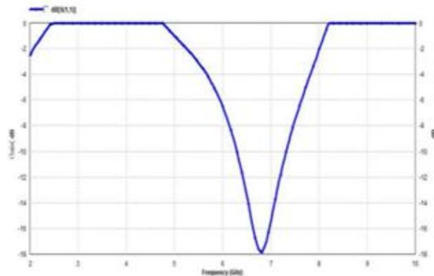
Figure.3. Return loss of proposed patch antenna 1
