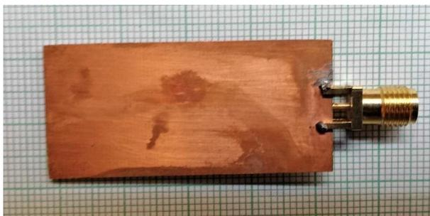
**Figure.7.(b): A Snapshot of Fabricated Antenna Bottom View**
