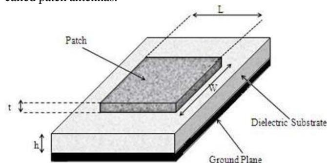
**Figure.1. Basic Structure of a Patch Antenna**
