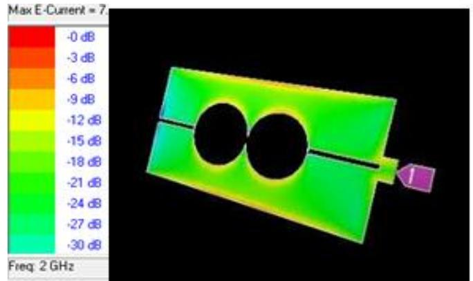
**Figure.8. Current distribution of proposed patch antenna 2**
