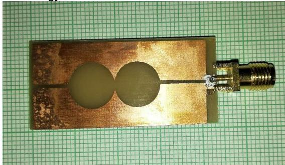
**Figure.7.(a): A Snapshot of Fabricated Antenna Top View**
