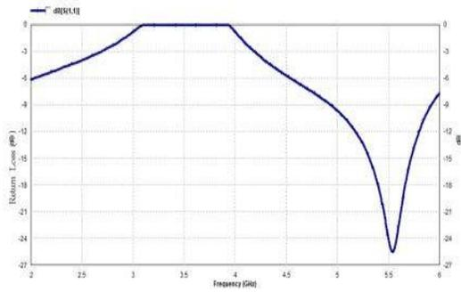
**Figure.6. Return loss of proposed patch antenna 2**
