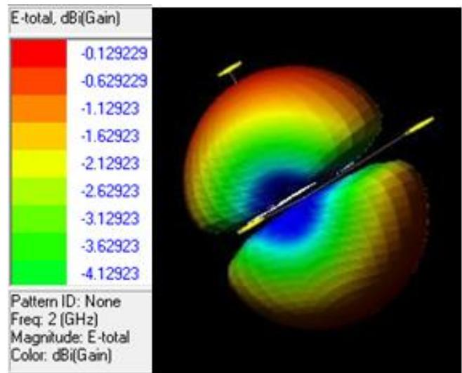
**Figure.9. Radiation Pattern of proposed patch Antenna 2**
