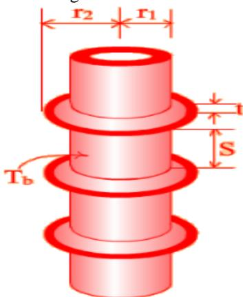
Figure.6.3 Circular Fins Mounted on Aluminum Cylinder
