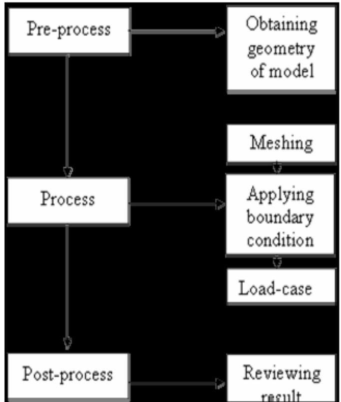
**Figure.3.Typical CFD procedures by commercial software**
