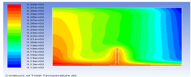
Figure.7. Contours of Total Temperature For Tube With Single Rectangular Fin
