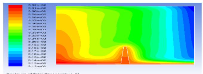
Figure.8. Contours of Total Temperature For Tube With Single Trapezoidal Fin
