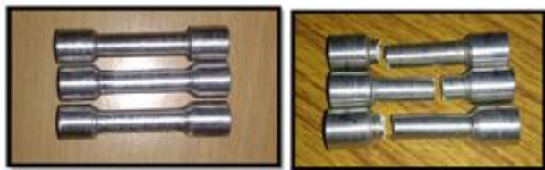
Figure 4.2. Tensile Specimens Before and After Test
