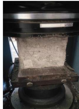
**Figure.3. Compression Testing Of Cube**
