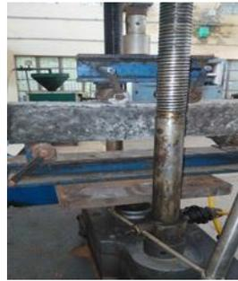
Figure.7. Flexure Strength Testing Of Small Beams
