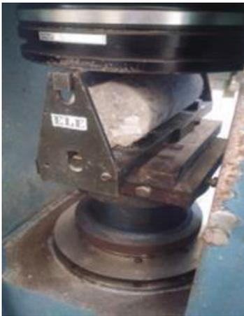
Figure.5. Split Tensile Testing Of Cylinder
