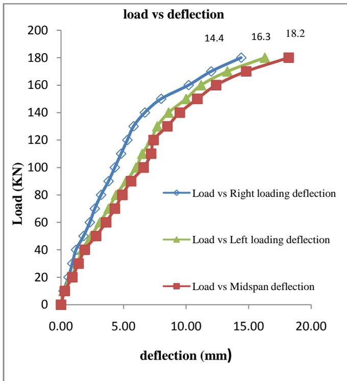
**Figure.4a. Load v/s deflection curve for control beam**
