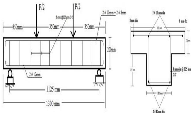
Figure.1. Beam reinforcement details
