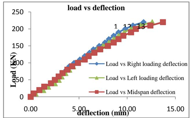
Figure.4f. Load v/s deflection curve for GSDL specimen
