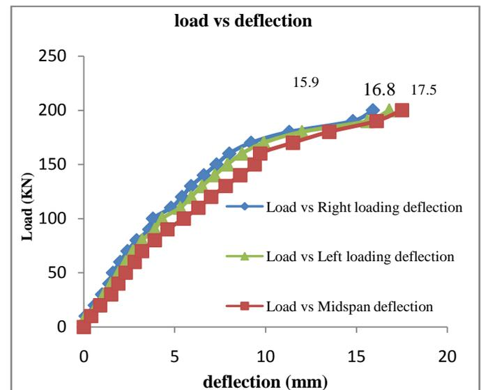
**Figure.4c. Load v/s deflection curve for BSSL specimen**
