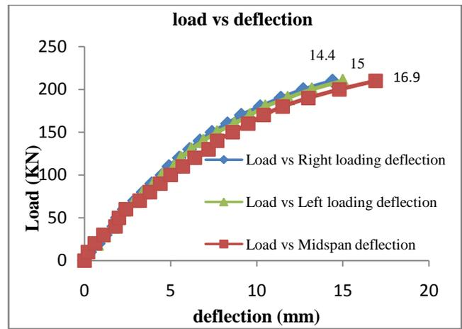
**Figure.4b. load v/s deflection curve for PT-CB specimen**
