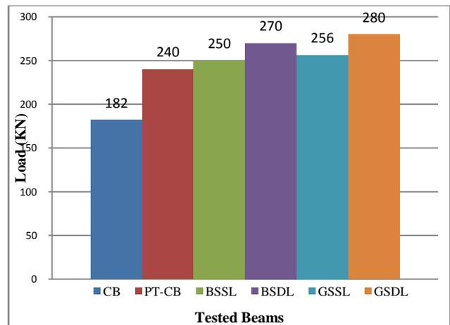
Figure.5. ultimate load of various beams
