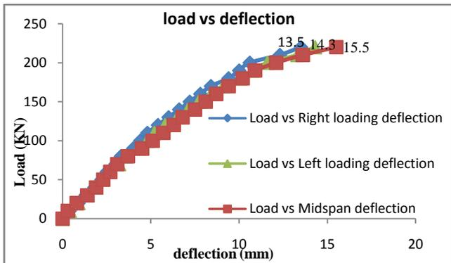
Figure.4d. Load v/s deflection curve for BSDL specimen
