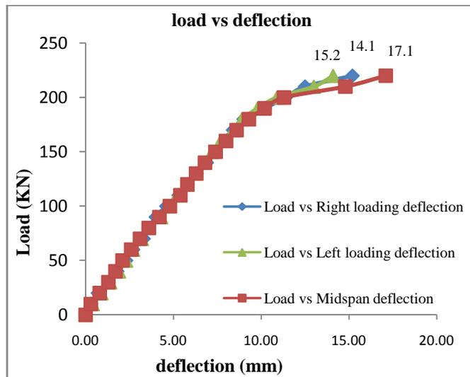
Figure.4e. Load v/s deflection curve for GSSL specimen
