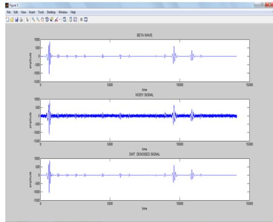
**Figure.4. Signal Decomposition And Denoising Of Beta Wave**
