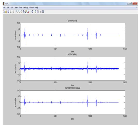
**Figure.5. Signal Decomposition And Denoising of Gamma Wave**
