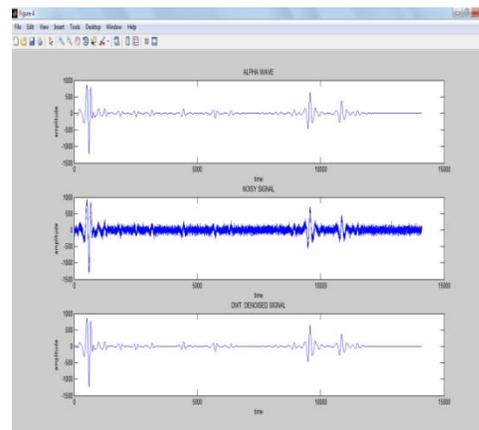
Figure.3. signal decomposition and denoising of alpha wave.
