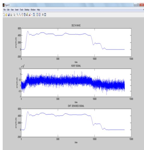
**Figure.6. Signal Decomposition and Denoising of Delta Wave**
