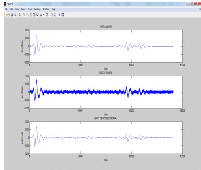
**Figure.7. signal decomposition and denoising of theta wave.**
