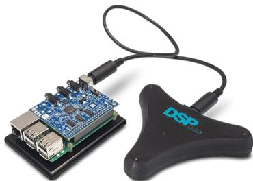
Fig. 2.3 HD DSP board with dual -core DBMD5
