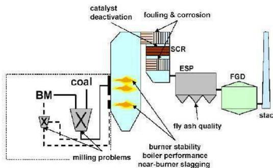
Figure.4. Direct Co-firing system
