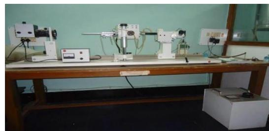
**Figure.13. Leitz Heating Microscope**
