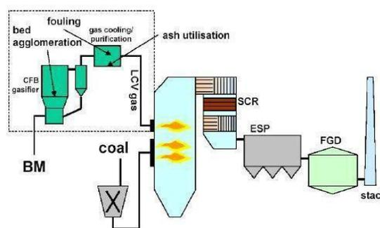
Figure.5. Indirect Co-firing system
