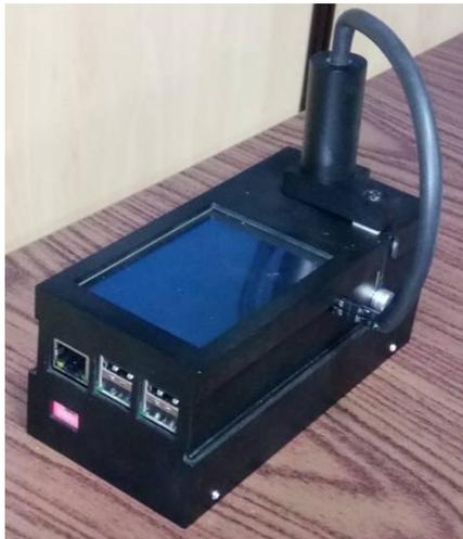
**Figure.5. Chlorophyll meter device developed.**
