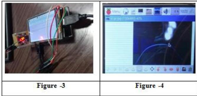
With the help of jumper wires the device is tested for its conceptual workflow. Figure – 3 shows the testing of the camera with the LED as light source. Figure -4 shows the image captured of NIR Light source (LED) which can only be detected by NIR camera Detector.
