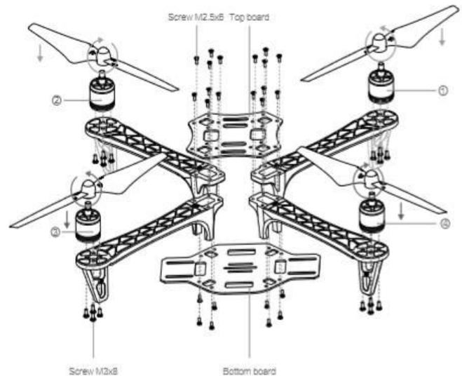
**Figure.7. assembling of quadcopter**
