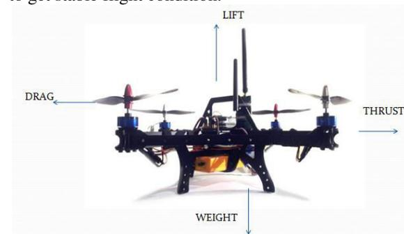
**Figure.1. Forces acting on quadcopter**
