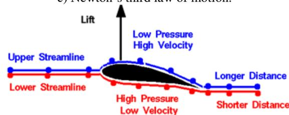
Figure. 3. Concept of lift
