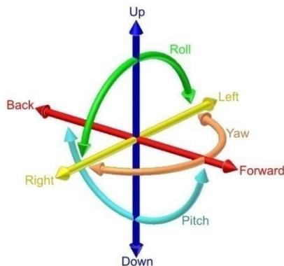
Figure.2. Axis of quadcopter
