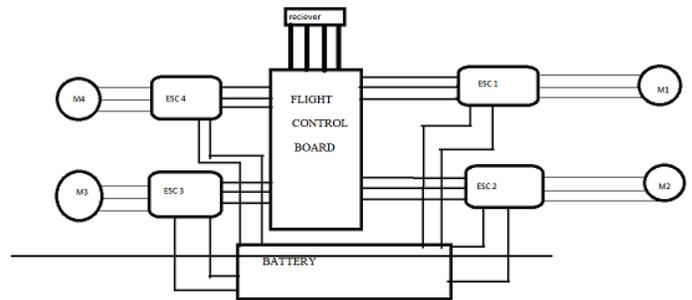
**Figure. 6. Circuit connections**
