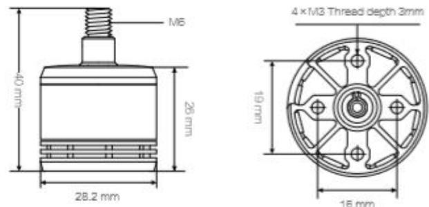
Figure.4. design of motor
