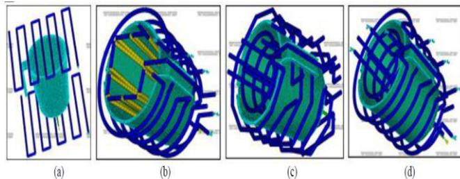
**Figure.5. Cooling Channel Types: (A) Normal, (B) Conformal Combination With Baffle, (C) Conventional Combination With Conformal And (D) Conformal**
