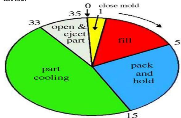
**Figure.4. Cycle Time In Injection Moulding**
