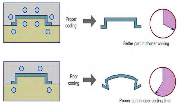
**Figure.1. Proper Cooling Design Versus Poor Cooling Design**
