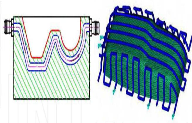
**Figure.2. A Layout Of Conformal Cooling Channels**
