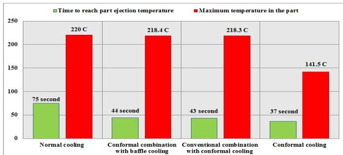
**Figure.6. Comparison of Time Reach Ejection Temperature and Maximum Temperature**
