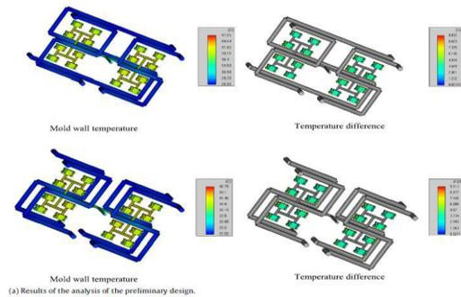
**Figure.3. Results of the C-Mould Cooling Analysis of the Preliminary Design**
