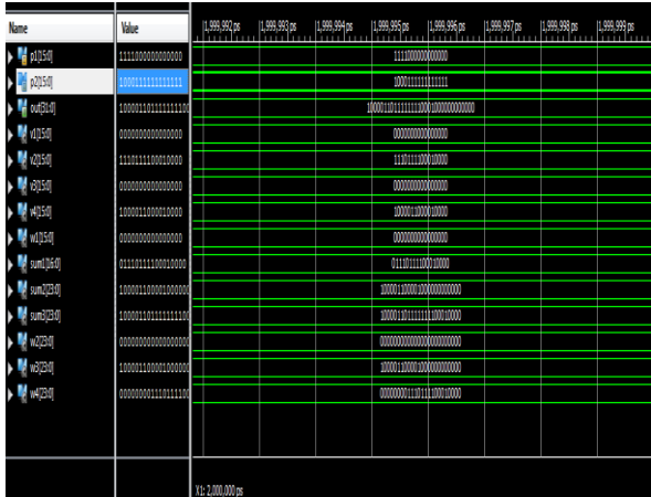
Figure 7: Simulation Result of 16X16 bitVedic Multiplier using Mux based adder using Brent Kung adder
