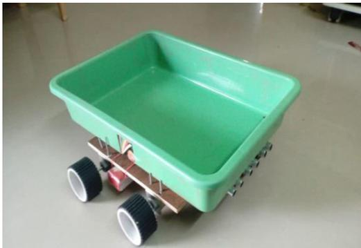
**Figure.5. Prototype of Design and Fabrication of Innovative Trolley Using Ultrasonic Sensor.**
