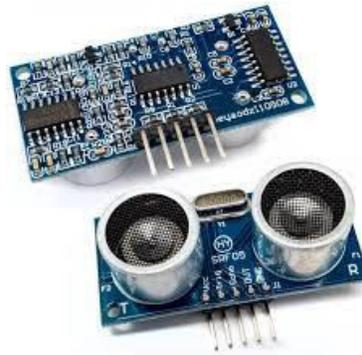
**Figure.2. Ultrasonic Sensor**
