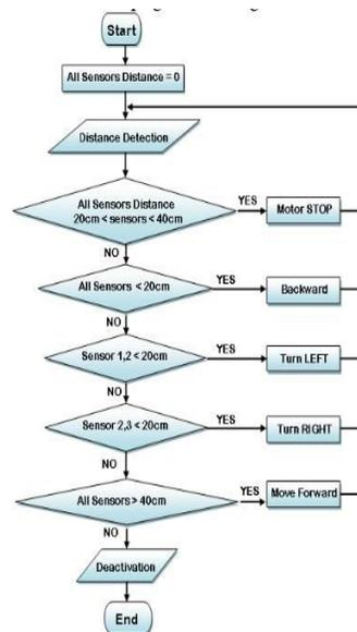
**Figure.4. Flowchart of Automatic Trolley**
