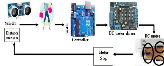
**Figure.3. Block Diagram of Automatic Trolley**
