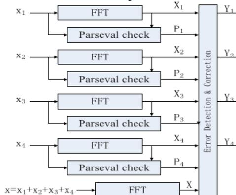
Figure. 2. Parity-SOS (first technique) fault-tolerant parallel FFTs.
