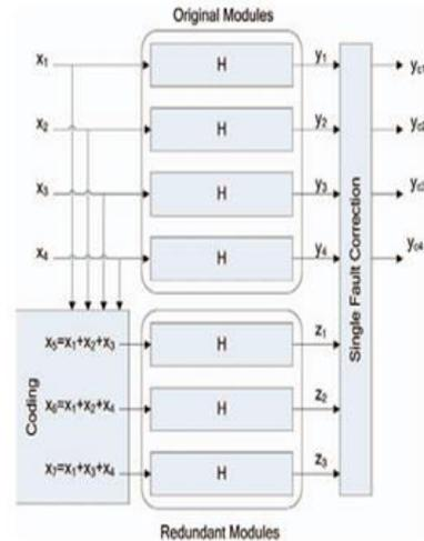
Figure. 1. ECC-based scheme for four filters and a Hamming code.
