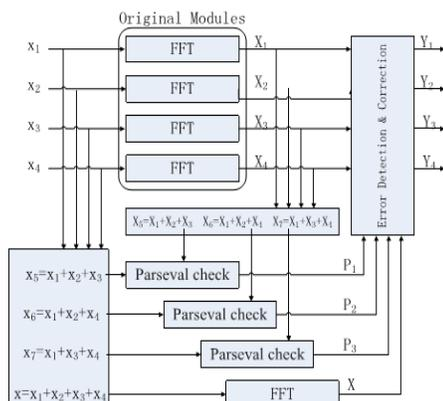
Figure 3. Parity-SOS-ECC (second technique) fault-tolerant parallel FFTs.
