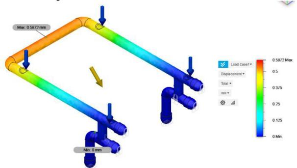
Figure.3. Displacement Diagram
