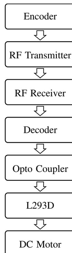
When the RF remote control is activated with programmed frequency, the load vehicle moves in the desired direction. It is also used to run the conveyor. As it is difficult to manually handle the machine that is partly submerged in the ditches, the remote control must be used for handling. When the function is over, a lever with hook is used to lift the machine.
