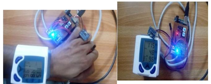
Figure.2. Implemented Wearable Health Monitoring Device
