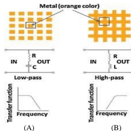
FIGURE 1. STRUCTURE OF FSS (A) PATCH TYPE FSS
