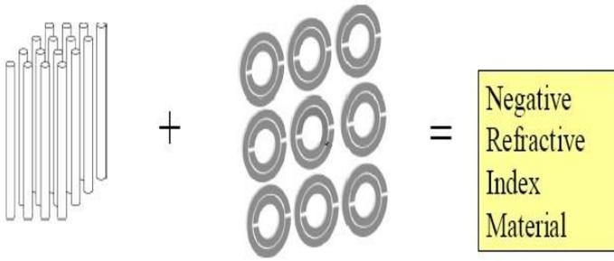
FIGURE 2: COMBINATION OF THIN WIRES AND SRR
