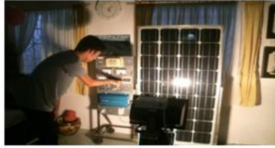
Figure 2. Student Monitor Voltage output using Floodlight
