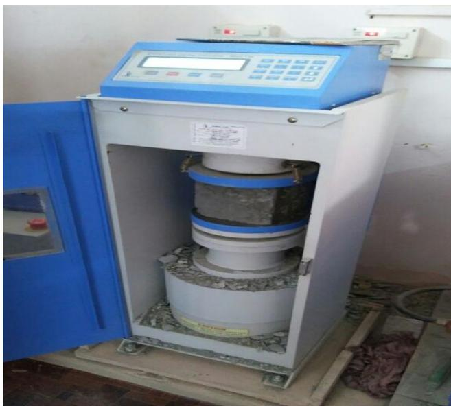
**Figure.5. Compressive strength testing of cubes casted with Pre-soaked SAP**
