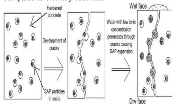
**Figure.1. Self sealing of cracks**
