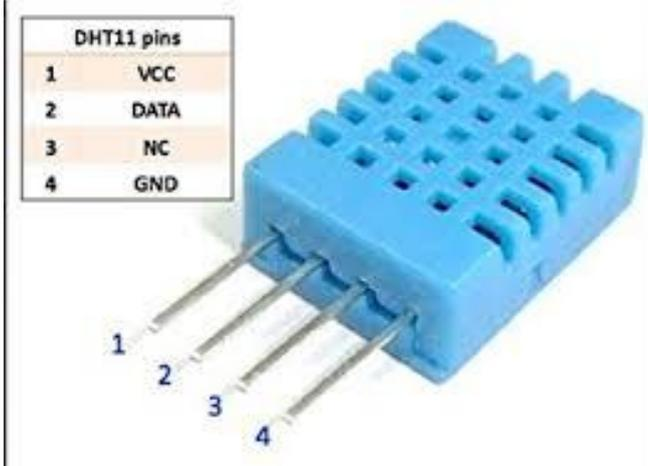
DHT11 is a Humidity and Temperature Sensor, which generates calibrated digital output. DHT11 can be interface with any microcontroller like Arduino, Raspberry Pi, etc. and get instantaneous results [1]. DHT11 is a low cost humidity and temperature sensor which provides high reliability and
