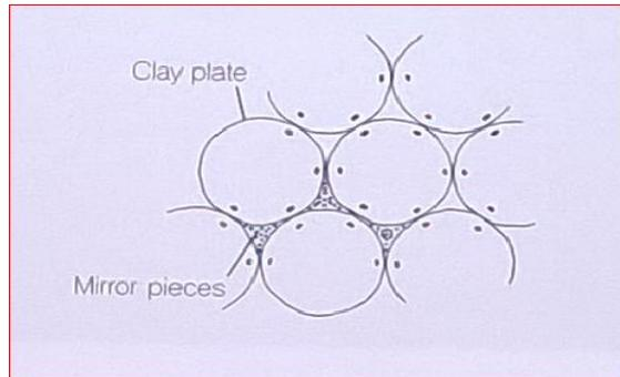
The local convex circular clay plates called tavdi are used for preparing rotis. These clay plates are claded on the external wall for insulation. Small holes are made in plates for ventilation and arranged in different designs and patterns. The
