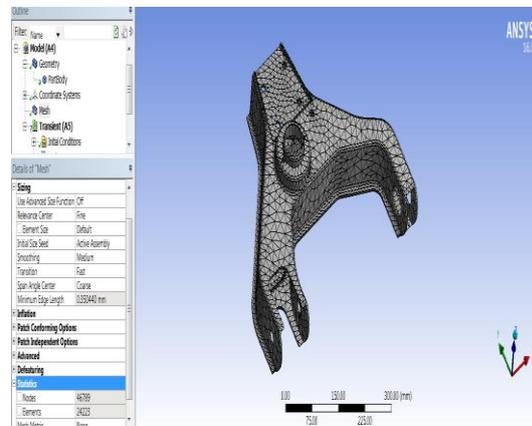
**Figure .6. Meshing of Upper Control Arm using Tetrahedral Element**
