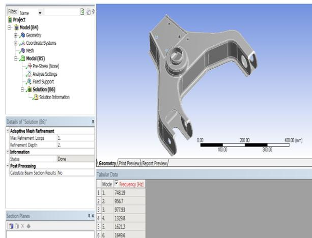
**Figure.9. Natural Frequency of Upper Control Arm**
