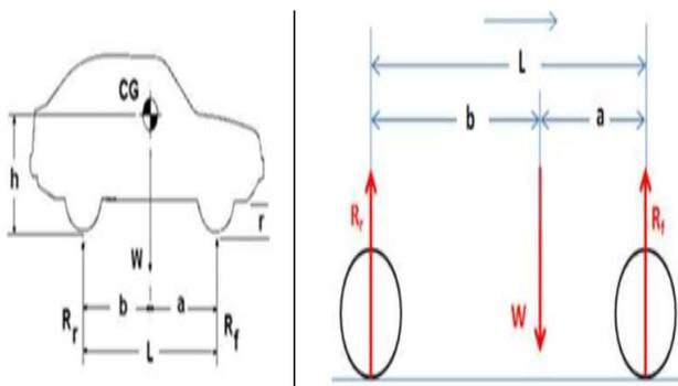
Figure.1. Forces on Stationary Car
