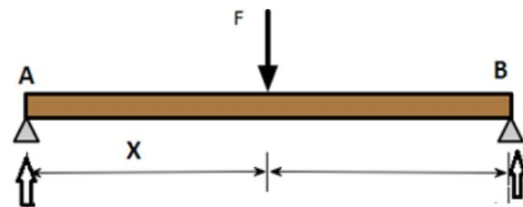
Figure.4. Force on the Axle Simply supported beam
