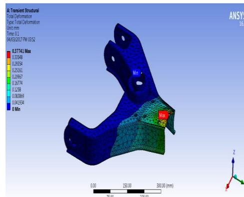
**Figure.8. Deformation of Upper Control Arm**
