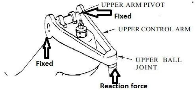
Figure.2. Boundary forces for Static Condition
