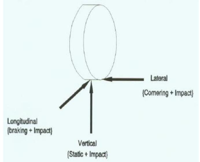
Figure.3. Wheel Loads and Directions
