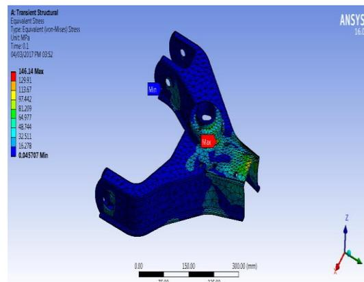
**Figure.7. Von Mises Stresses on Upper Control Arm**
