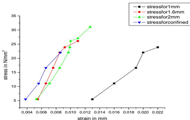
Graph No.3: Showing stress v/s strain behaviour of partially confined cage System for 1, 1.6 and 2mm thickness with 100mm spacing
