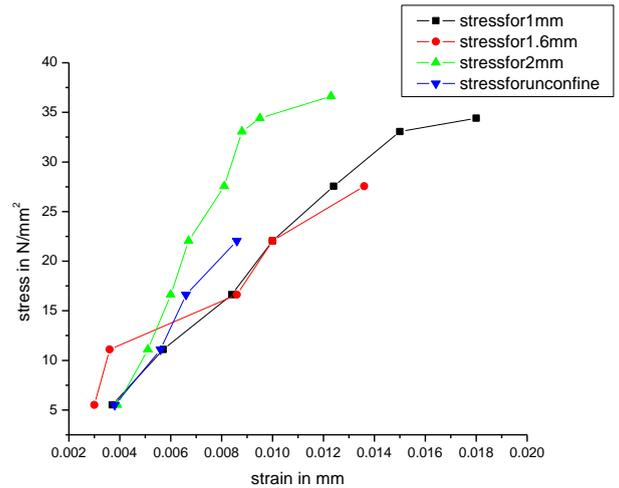
Graph No. 4: Showing stress and strain behaviour of partially confined cage system for 1, 1.6 and 2mm thickness and 50mm spacing
