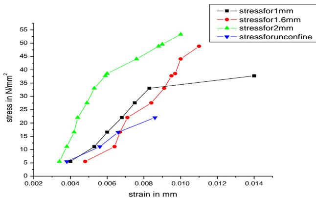
Graph No.2: Showing stress and strain behavior of partially confined cage system with thickness 1, 1.6 and 2mm thickness with 150mm spacing
