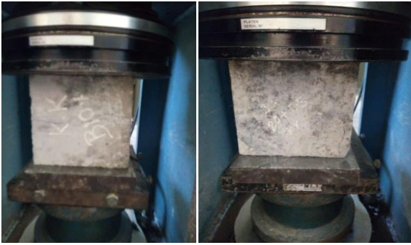
Figure.2. Testing of Cubes in Compression Testing Machine
