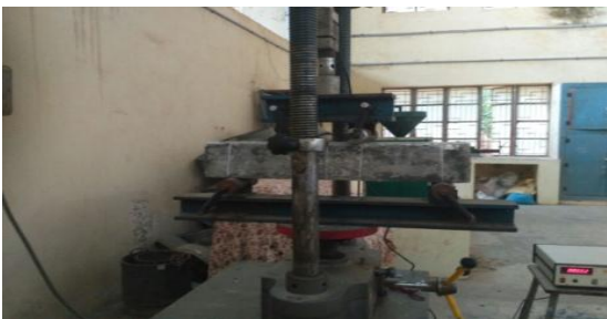
Figure.4. Flexure Strength Testing Of Prism
