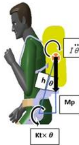
Figure.5. Stabilizing and destabilizing torques during motion
