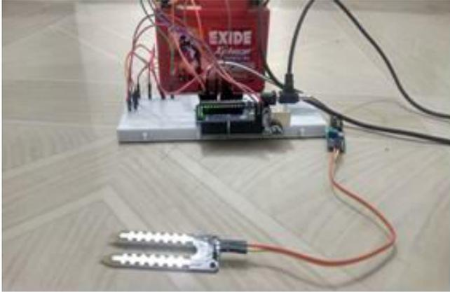
The connection for the Moisture sensor is a made with the help of the diagram above. the output is read through the analog pin A5 of the Arduino.
