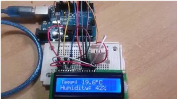
The connection for the LCD display is made through the I2C connection.i.e., Using SDA, SCL connection lines with the help of LCD I2C module and all the sensors are connected to the Arduino and the sketch is uploaded to get the value of temperature and moisture in the lcd display.
