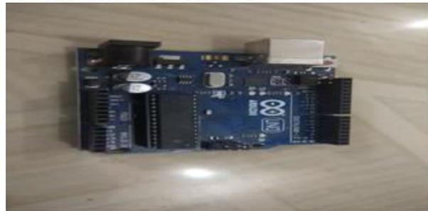
The Arduino uno board is a microcontroller based on the ATmega328. It has 14 digital pins in which 6 can be used as PWM outputs, a 16 MHZ ceramic resonator, an ICSP header, a USB connection, 6 analog inputs, a power jack and a reset button. The above given is the pin out configuration diagram for the Arduino unoR3. This is used as a reference to connect sensors to the system.
