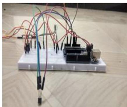
The first pin of the LM35 temperature sensor is connected to the 5v supply of the Arduino uno, the center pin is used for output and it is connected to the A0 analog reader pin for measurement purpose. The last pin is connected to the ground of the Arduino. Now, the output can be found in the serial monitor of the Arduino software after uploading the sketch.
