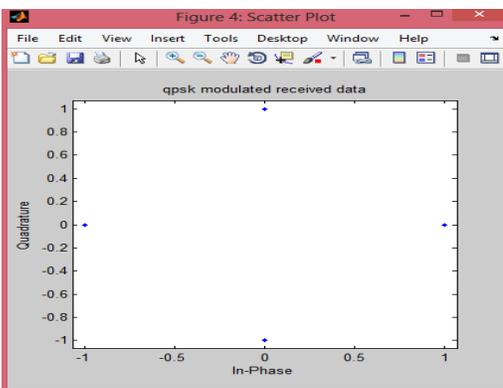
Figure.5.QPSK modulated received data represented in terms of In-phase and quadrature
