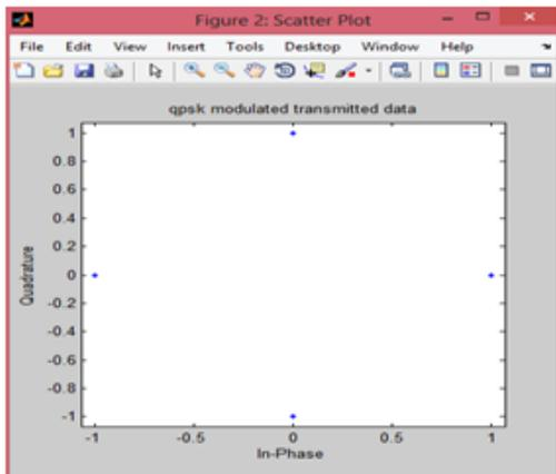
Figure.3.QPSK modulated transmitted data represented in In-phase and quadrature
