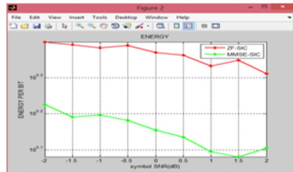
**Figure.9. Energy versus SNR in terms of ZF-SIC and MMSE-SIC**
