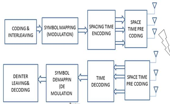
Figure.7.Block diagram for MIMO
