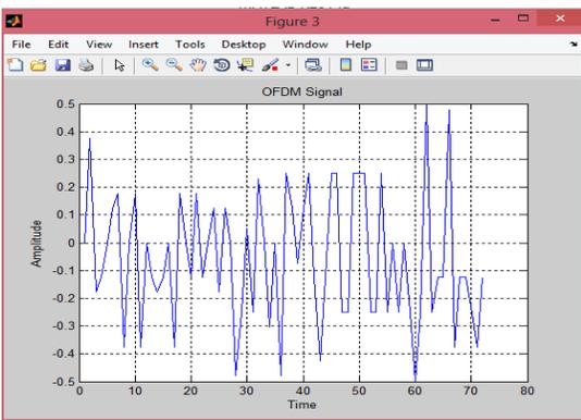
Figure.4.The OFDM signal generated for the given 64 bits data
