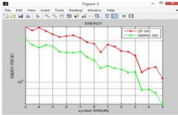
Figure.12.The Energy per bits for SNR Ranges from -5 to 5.
