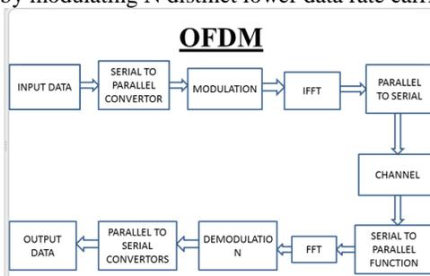
Figure.1. Block diagram for OFDM
