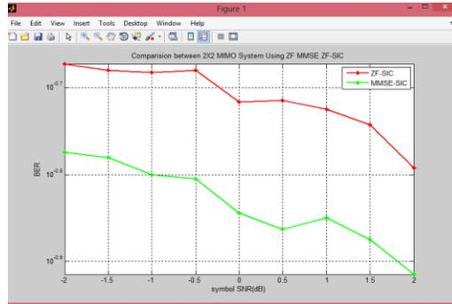
**Figure.8.2x2 MIMO system using ZF-SIC and MMSE-SIC**
