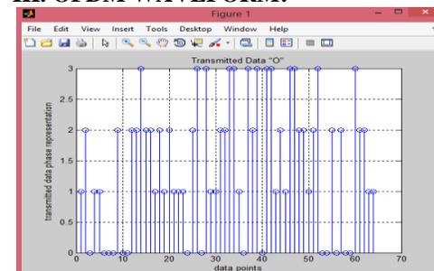
Figure.2. The transmitted data phase representation of 64 bit input data
