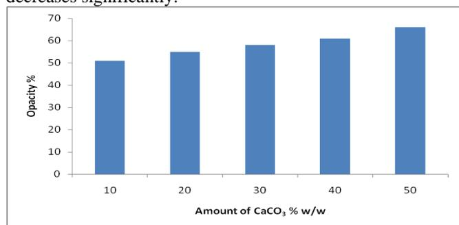
**Figure.8.** Showed the effect of  $\text{CaCO}_3$  nanoparticles on the opacity of PSBBCCF
