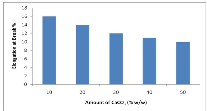
Figure.4. showed the effect of CaCO<sub>3</sub> nanoparticles in elongation at break
