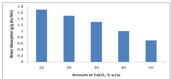
Figure.7. Showed the effect of CaCO<sub>3</sub> on the water absorption capacity of PSBBCCF
