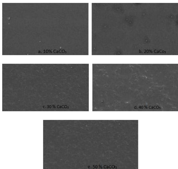
**Figure.10.** Showed SEM images of sample a, b, c and d having 10%, 20 %, 30%, 40% and 50%  $\text{CaCO}_3$  in PSBBCCF respectively.
