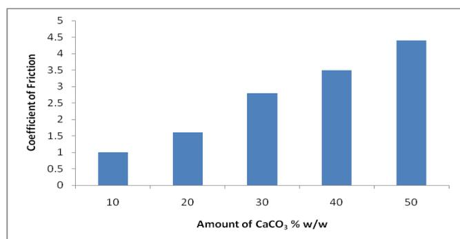
**Figure.9.** Showed the effect of  $\text{CaCO}_3$  on the coefficient of friction of PSBBCCF
