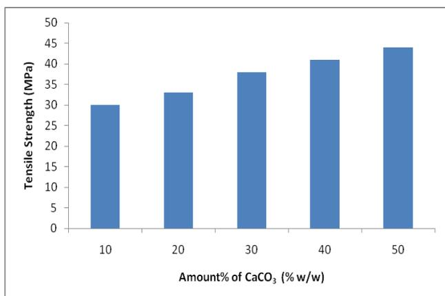
Figure.3. Showed the effect of CaCO<sub>3</sub> nanoparticles on the tensile strength of PSBBCCF
