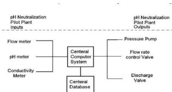
**Figure.1. Block Diagram Of System**
