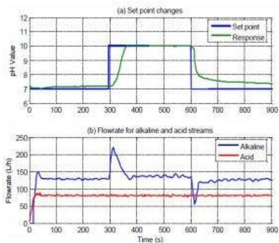
**Figure.3. Performance of combination control mechanism.**
