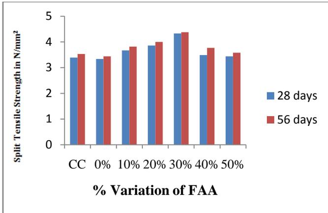
Figure.8. % Variation of FAA With Respect To NCA for 28 And 56 Days in N/Mm<sup>2</sup>
