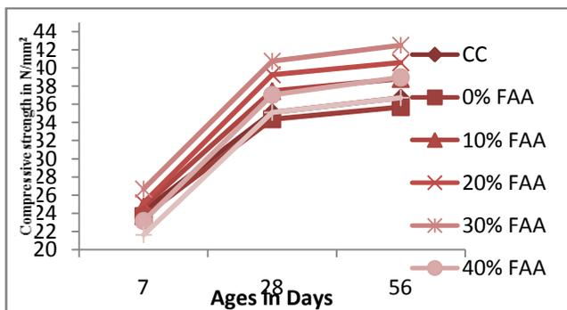
Figure.7.% Variation of FAA With Respect To NCA for 7 And 28 Days in N/Mm<sup>2</sup>
