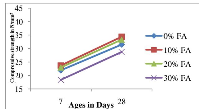
**Figure.3. % Variation of Fly Ash With Respect To Cement for 7 And 28 Days in N/Mm<sup>2</sup>**
