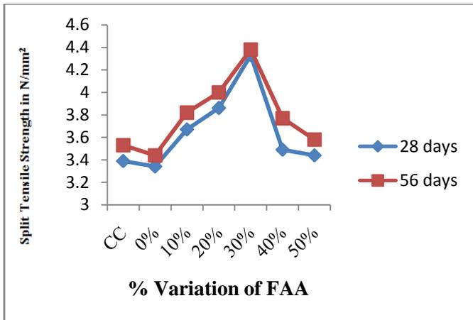
Figure.9. % Variation of FAA With Respect To NCA for 28 And 56 Days in N/Mm<sup>2</sup>
