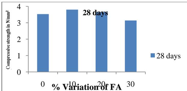
**Figure.4. % Variation of Fly Ash With Respect To Cement for 28 Days in N/Mm<sup>2</sup>**
