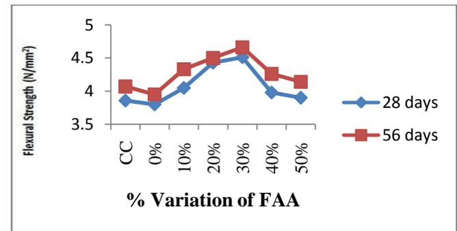
Figure.12. % Variation of FAA With Respect To NCA for 28 And 56 Days in N/Mm<sup>2</sup>
