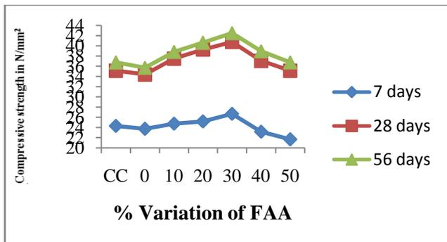
Figure.6. % Variation of FAA With Respect To NCA for 7 And 28 Days in N/Mm<sup>2</sup>
