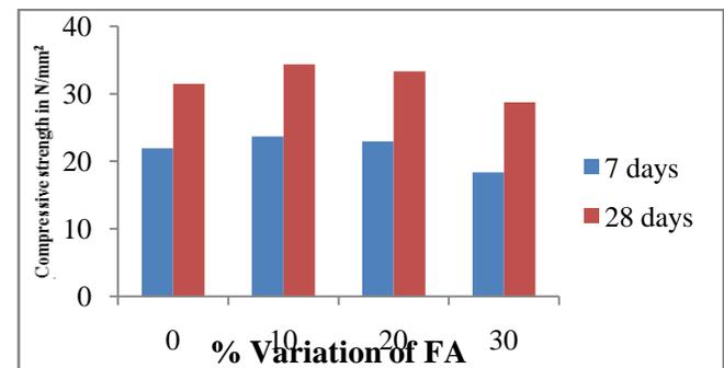
**Figure.2. % Variation of Fly Ash With Respect To Cement for 7 And 28 Days in N/Mm<sup>2</sup>**
