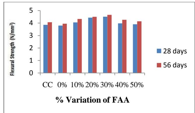
Figure.11. % Variation of FAA With Respect To NCA for 28 And 56 Days in N/Mm<sup>2</sup>
