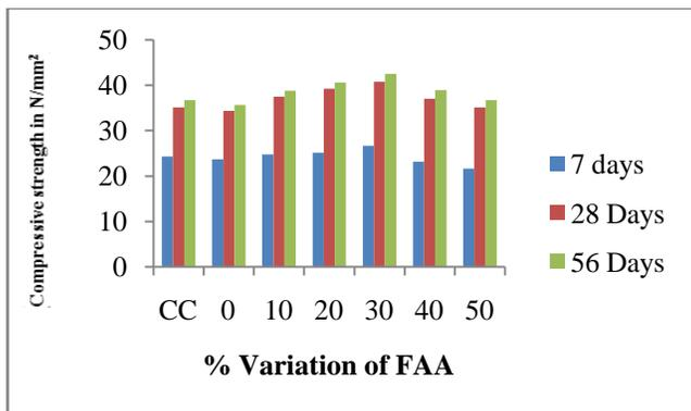
Figure.5. % Variation of FAA With Respect To NCA for 7 And 28 Days in N/Mm<sup>2</sup>
