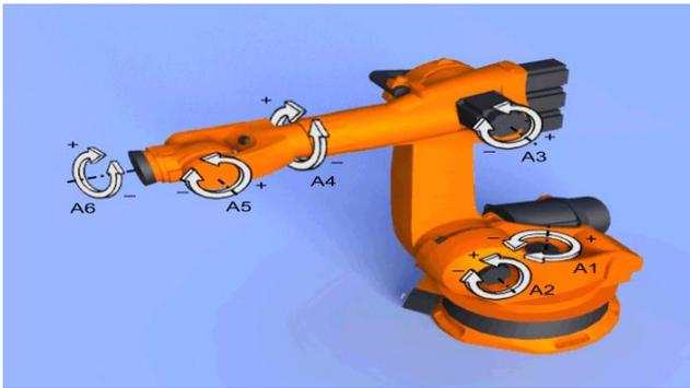
Figure.5. Axis Specific co-ordinate system
