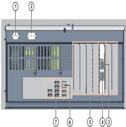
**Figure.15. Motherboard D2608-K interfaces**
