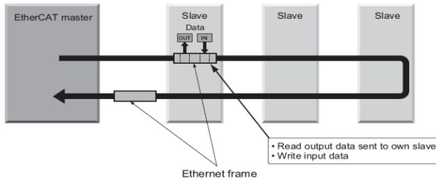
Figure.19. Ether CAT Mechanism
