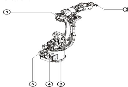
**Figure.4. Connecting cables and interfaces**
