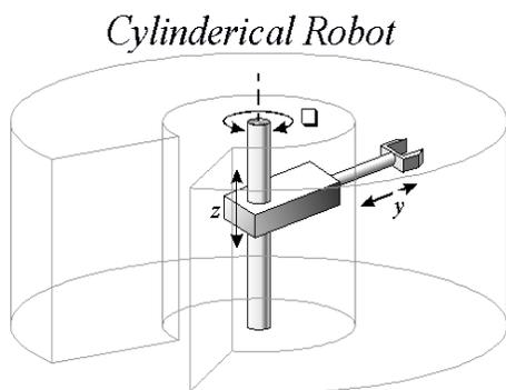
Figure.7. Cylindrical coordinate system
