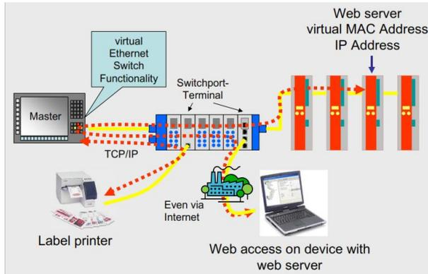
Figure.21. Ethernet over EtherCAT
