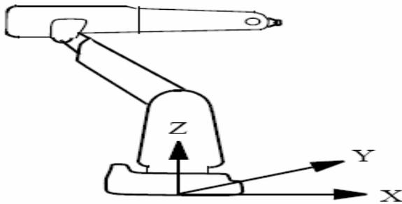
Figure.6. Base coordinate system of a manipulator
