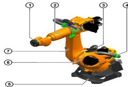
**Figure.1. Overview of Manipulator components**
