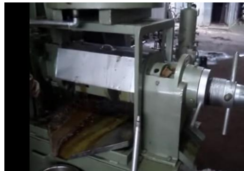
Figure.4.1 Eucalyptus and Madhuca longifolia oil Seed crushing machine
