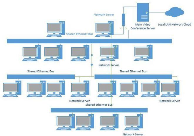
**Figure.7. Proposed Star-Bus hybrid (4x4=16 network nodes, where N=4, S=1, a=4) Topology for real time (video conference) high-speed data transfer following M/M/1 queuing theory**
