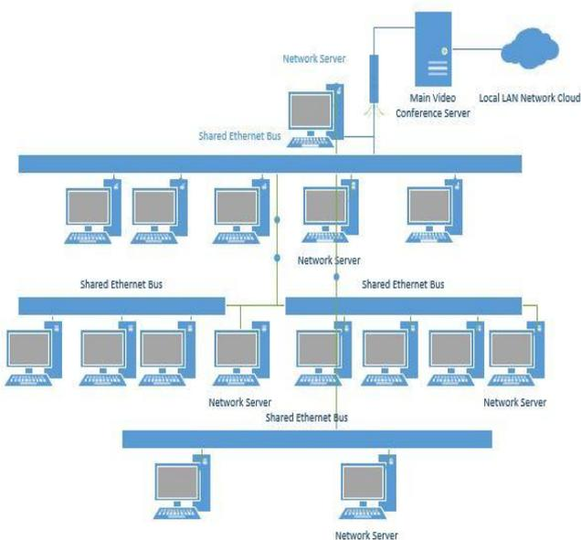
Figure. 5. Distributed System Networks (Minicomputer model architecture)
