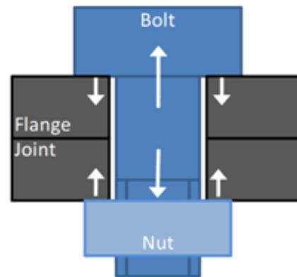
Figure 2: Bolted Joint Clamping Forces
