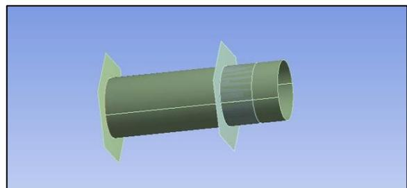
Figure.7. Nut and bolt section model used for application of composite layers
