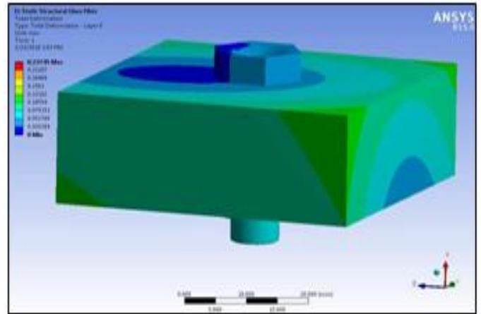
Figure.9.: Maximum displacement in whole assembly of 0.2374 is observed
