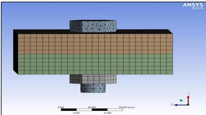
Figure.5. Meshing of Nut and bolt
