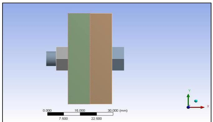
**Figure.3. Bolted lap joint**
