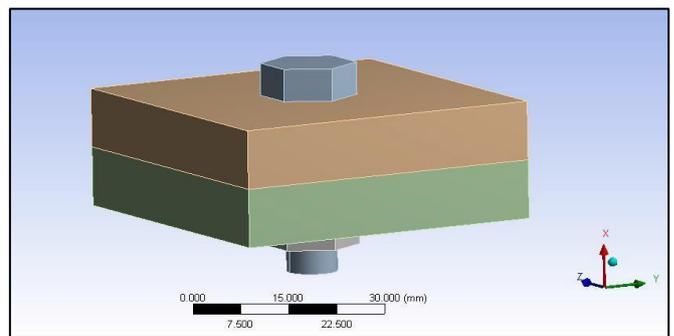
**Figure.2. Bolted lap joint**
