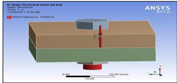
Figure.6. Bolted lap joint assembly with applied forces and boundary conditions
