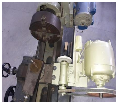
Figure.9. Installed Turnery Nexus on 2-Super Lathe Machine
