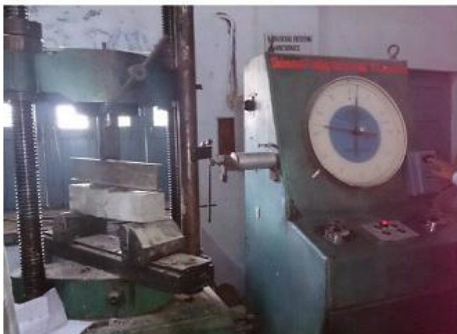
Figure. 3. Failure Pattern and Test Setup for Flexural Loading
