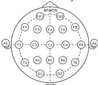
Figure. 1. 10-20 Electrode Cap
