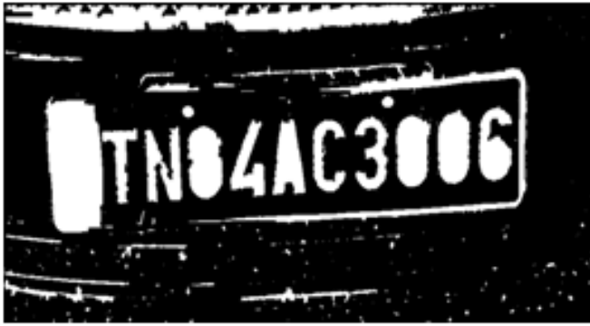
Figure.6 Image after removing noise & filling holes
