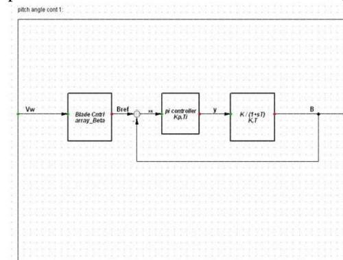
Figure 8.1 Pitch angle block
