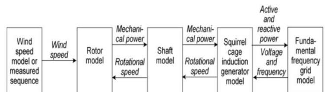
**Figure.2.1 Block Diagram of Wind Energy Conversion System**
