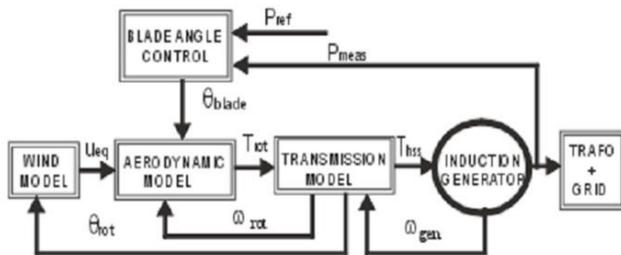
Figure 5.1 General Structure of fixed speed wind electric system
