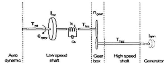
Figure 7.1 Drive train model of two mass shaft
