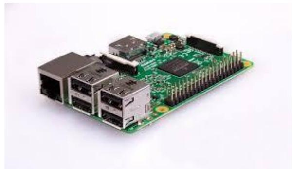
FIG. 4. RASPBERRY PI FOR COMMUNICATION AND PROCESSING
