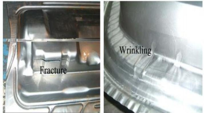
**Figure.1. Fracture and Wrinkling faults in the forming process**
