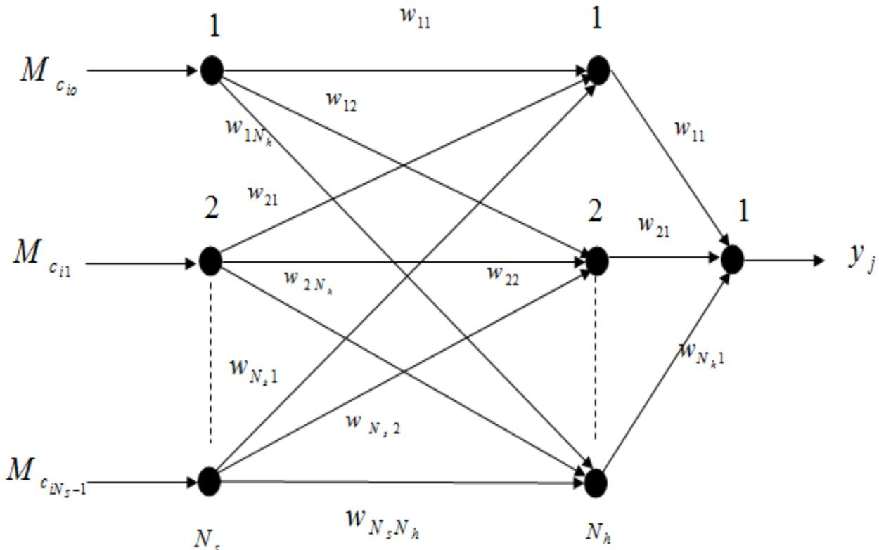
Figure.4. N Inputs and One Output Neural Network to Train the Dataset
