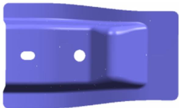
**Figure.2. Automobile inner panel**
