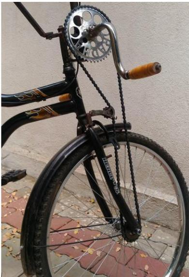
**Figure.3. Sprocket Chain Setup**
