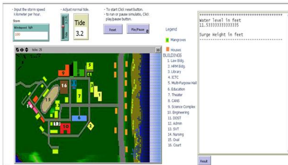
Figure.5. Screenshot of Simulation Output on the affected properties/areas in 100 kph wind speed. 100 kph wind speed got 11.533333333333335 water levels in feet and no damageable objects.
