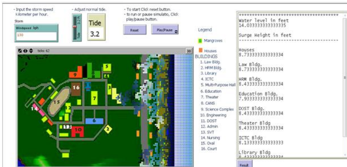
Figure 6. Screenshot of Simulation Output on the affected properties/areas in 130 kph wind speed. 130 kph wind speed got 14.033333333333335 water levels in feet and some damageable objects in infrastructures.
