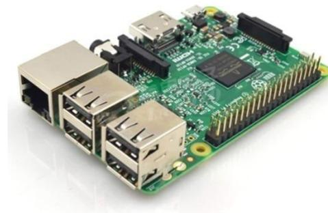
**Figure.1. Raspberry pi 3 Model B**
