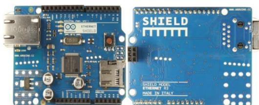
**Figure.9. Ethernet shield**
