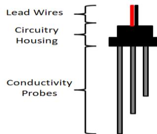
Figure.4. Electrical conductivity sensor
