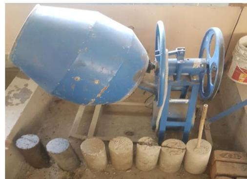
FIGURE 4: CONCRETE CYLINDERS
