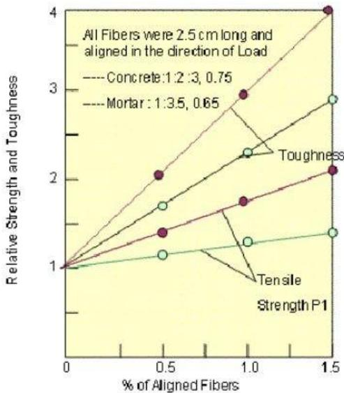
FIGURE 1: EFFECT OF VOLUME OF FIBERS IN FLEXURE [3]
