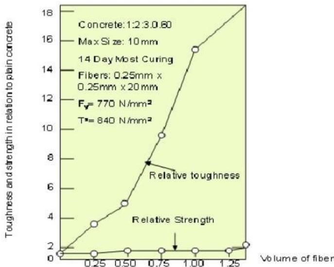
FIGURE 2: EFFECT OF VOLUME OF FIBERS IN TENSION [3]
