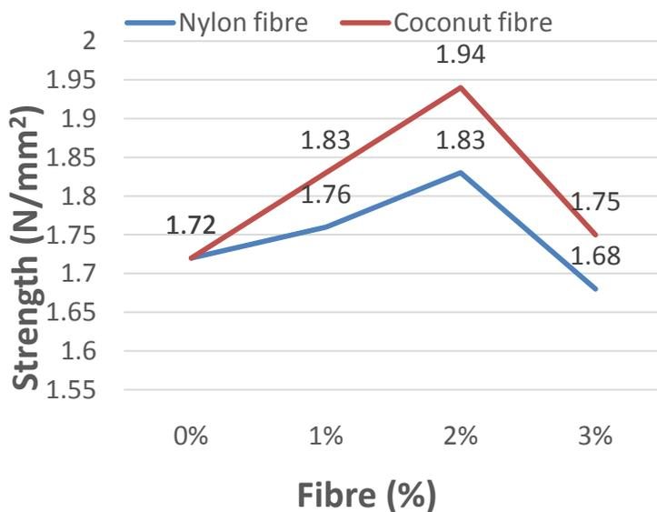
PLOT 2: COMPARISON OF RESULTS OF SPLIT TENSILE STRENGTH TEST COMPRESSION TEST RESULTS FOR NYLON AND COCONUT FIBER
