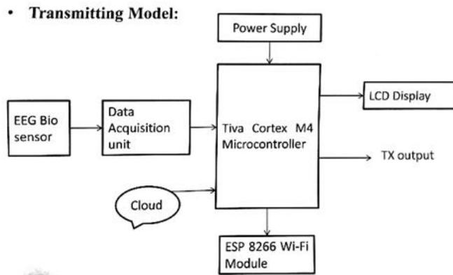
**Figure.1. Block Diagram of transmitting model**
