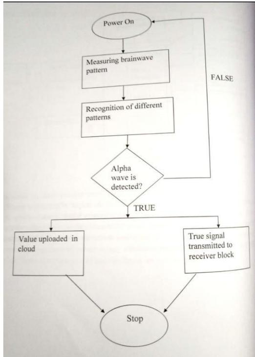
**Figure.3. Flow chart for Transmitting model**
