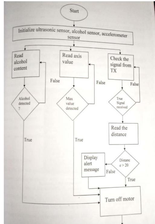
**Figure.4. Flow chart for Receiving model**
