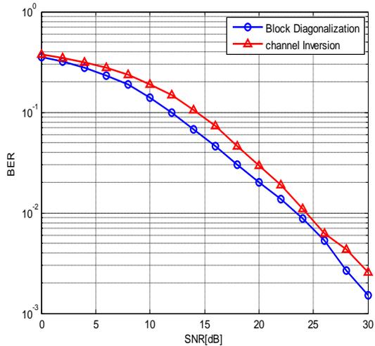
**Figure.3. BER versus SNR [dB] for linear precoding**
