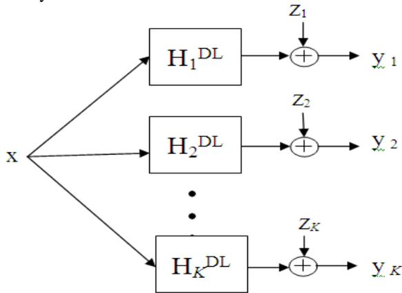
Figure.2. Downlink channel model for MU-MIMO
