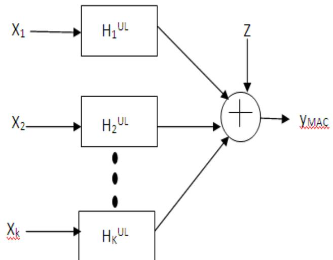
Figure.1. Uplink channel model for MU-MIMO [6]
