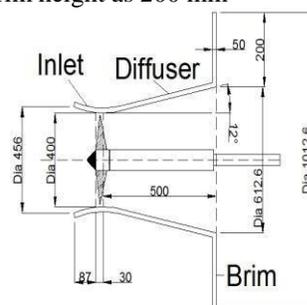
Fig 2. Reference model with thickness 50mm and brim height 200mm
