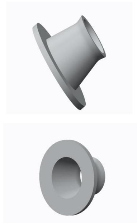
**Fig.24 3D views of Cylindrical Brimmed Diffuser Model**
