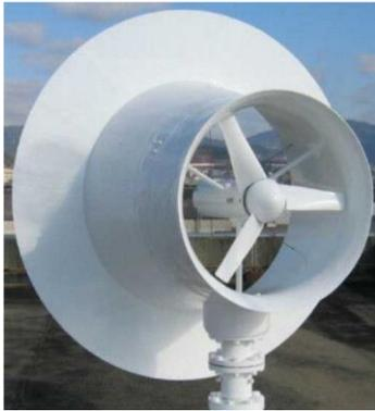
Fig.3 Cylindrical Brimmed Diffuser Wind Turbine (Small Wind Turbines)
