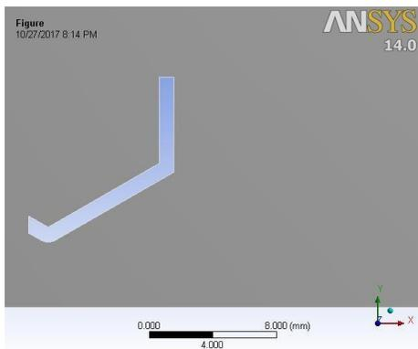
Fig.5: 2D Axisymmetric Model of Cylindrical Brimmed Diffuser
