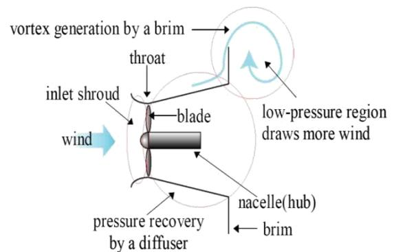
Fig.1 Principle of Cylindrical Brimmed Diffuser Wind turbine
