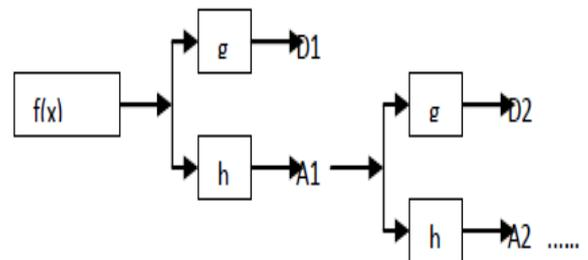
Figure 3 sub-band decomposition of a EEG signal by using Discrete Wavelet Transform
